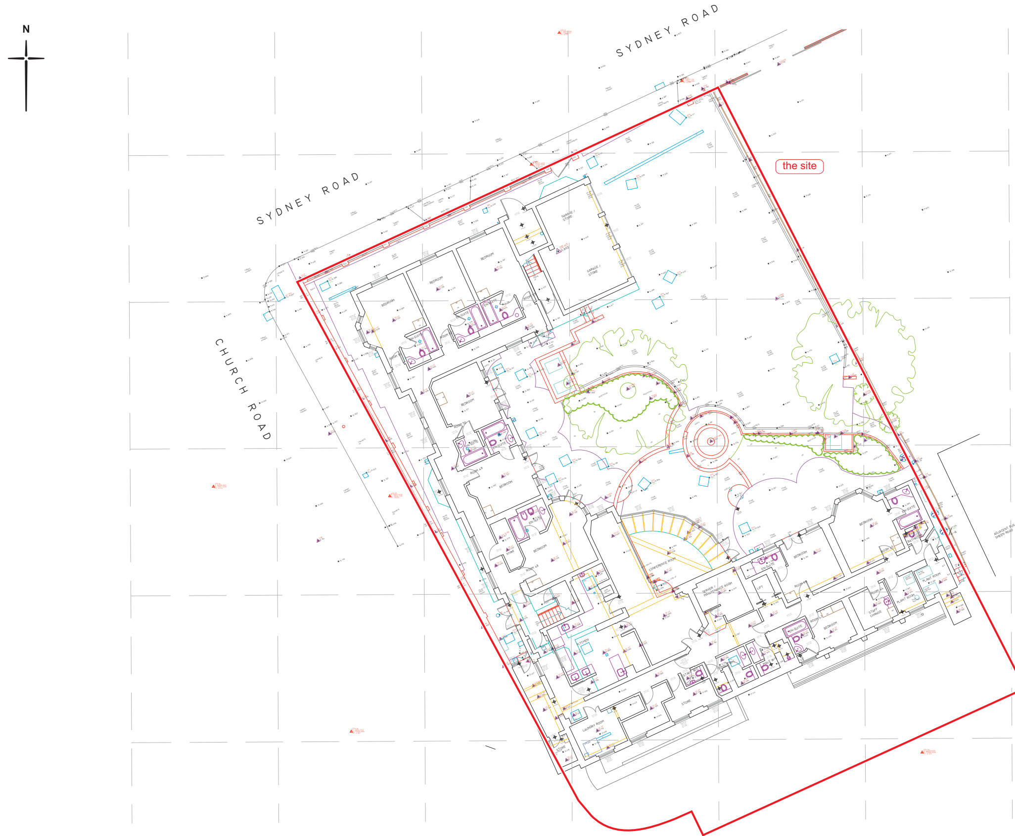
Fig 9 Plan of existing lower ground floor with levels (Mobile Cad Surveying Solutions, dwg no. 2844-02, August 2021)
