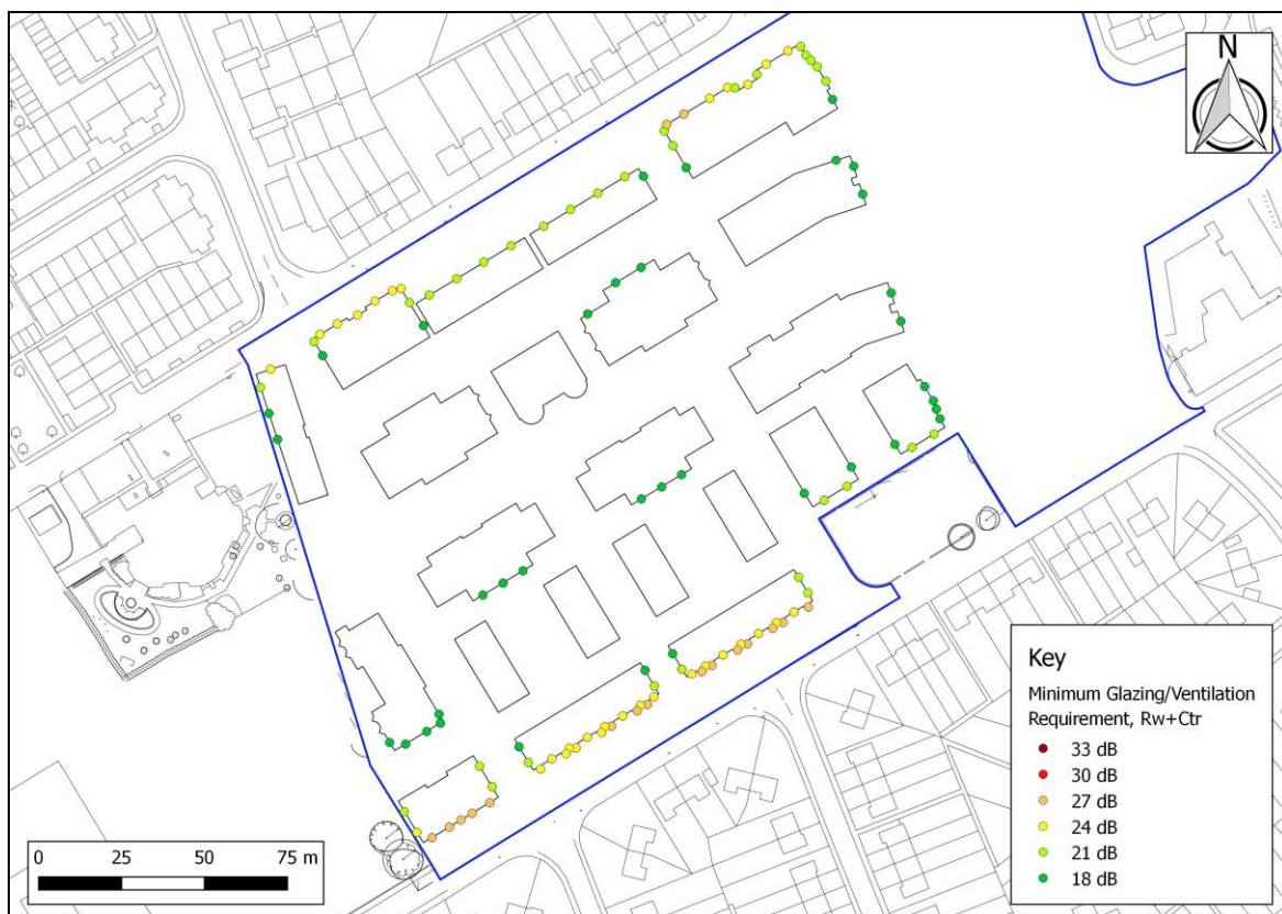
Figure 6.3 Glazing and Ventilation Requirements
