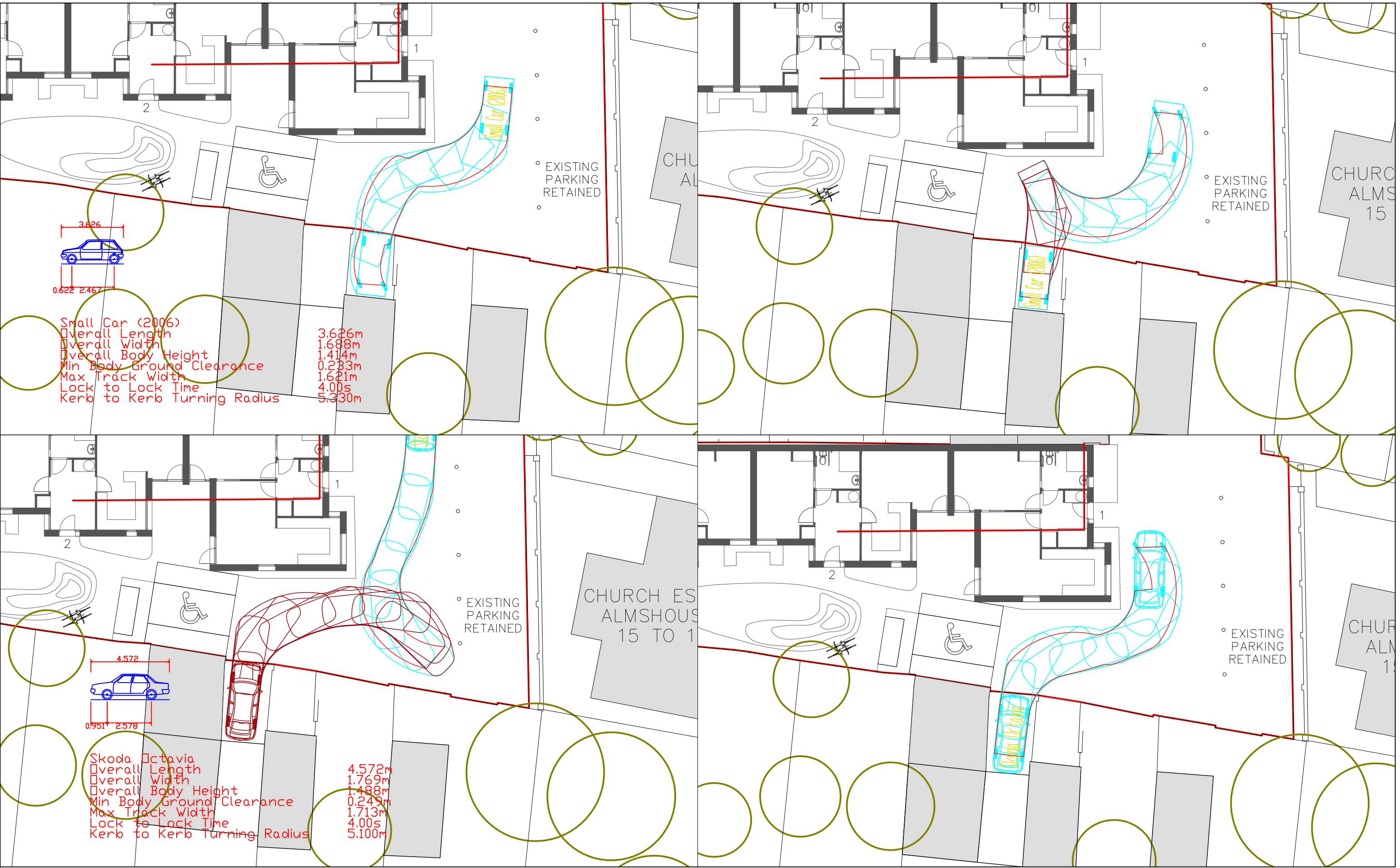
P2689: ST MARY'S GROVE GARAGES Figure 4.b Vehicle Swept Path Analysis: Car Accessing Existing Garages at numbers 13 and 15 Townsend Rd
