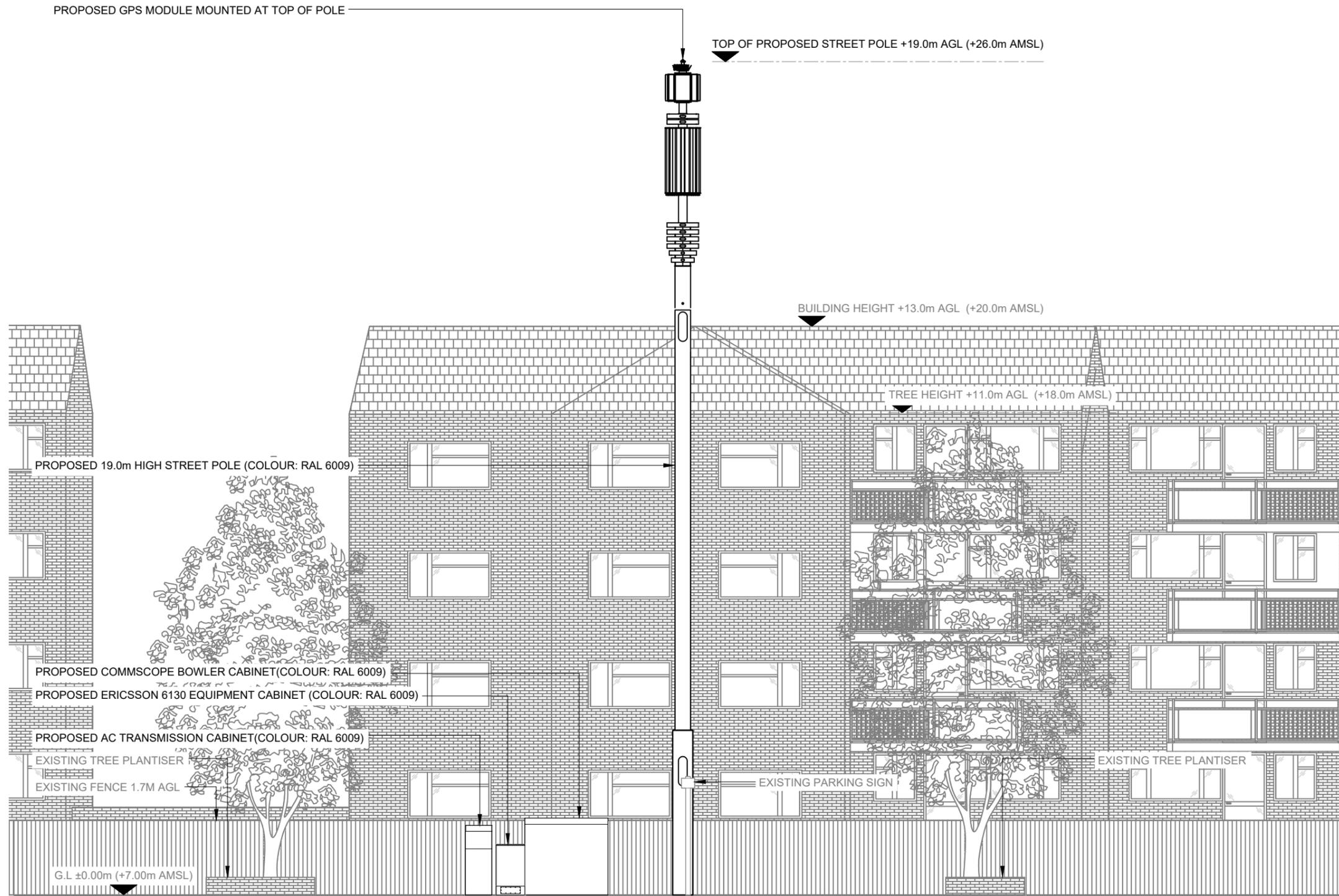
PROPOSED SITE ELEVATION A
