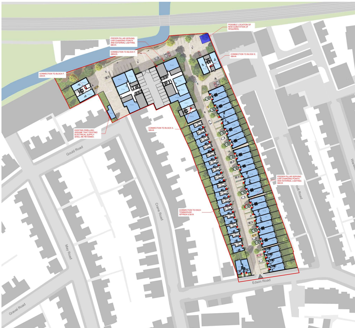
Indicative Substation Location and Meter Positions
