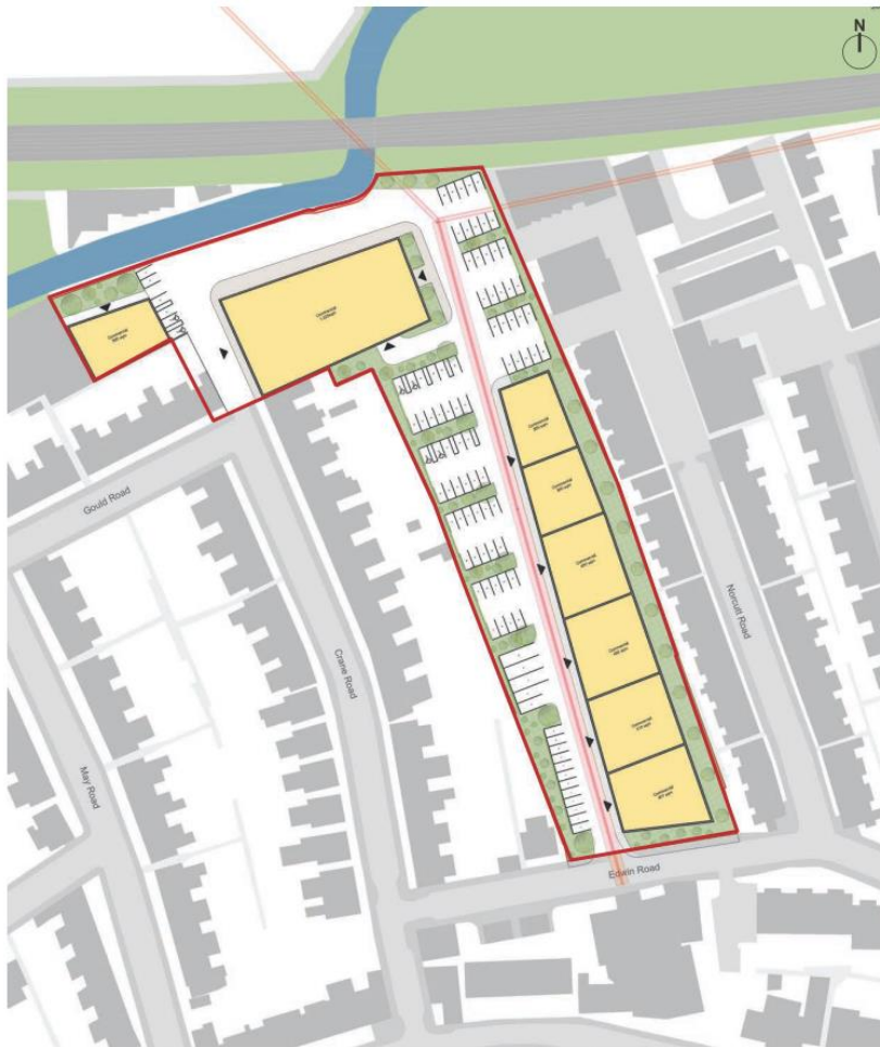
Ground floor plan of full industrial scheme of B1/B2/B8 uses achieving 3,773 sq m (1-3 storeys)
