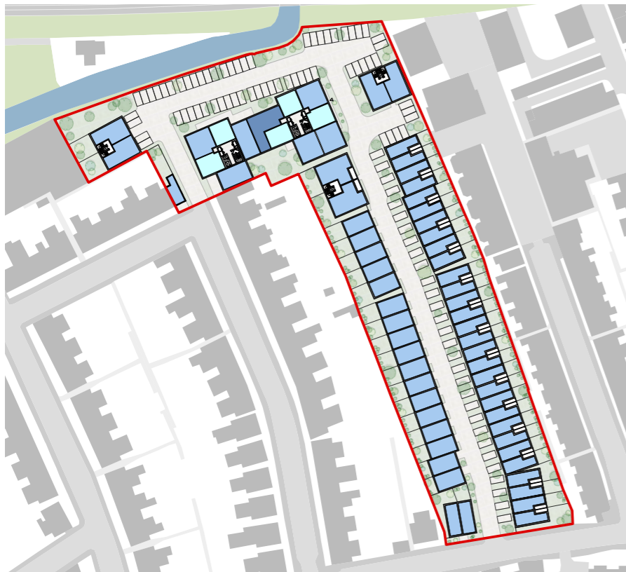
Initial layout showing four storey townhouses without internal car parks or garages
