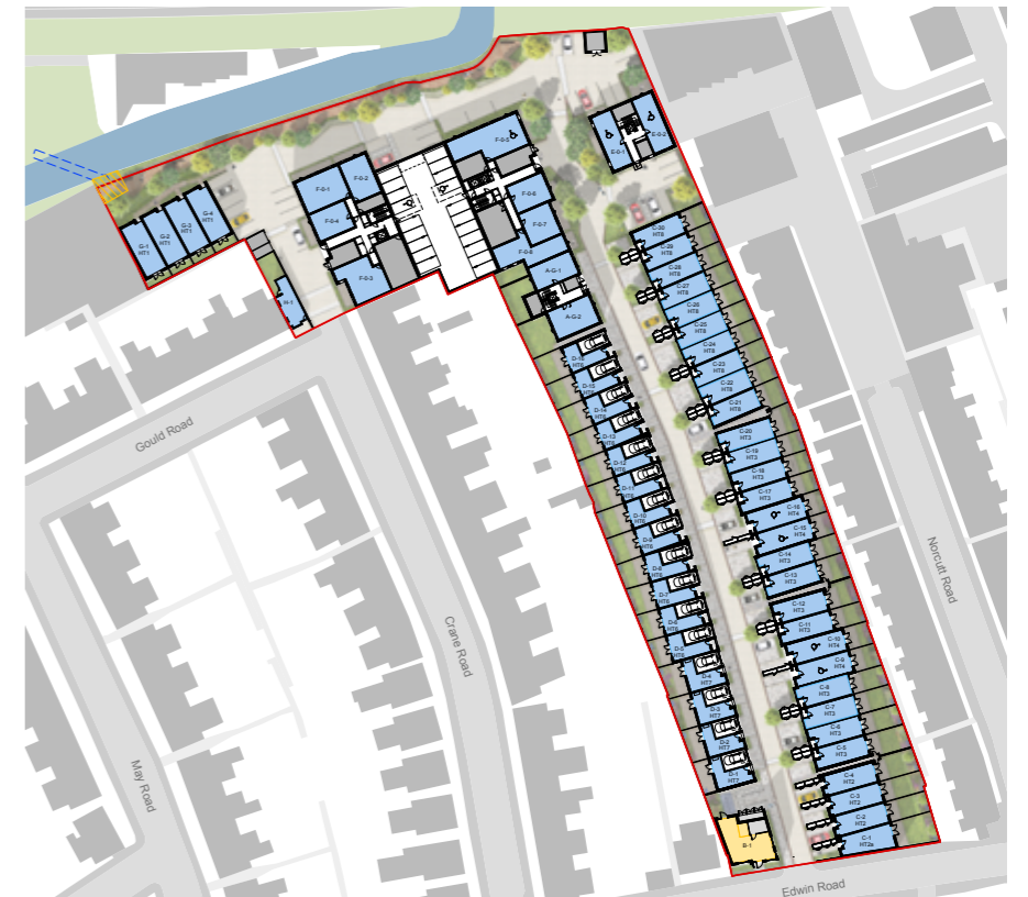
Layout adjusted for sewer line and to accommodate commercial (Use Class E)
