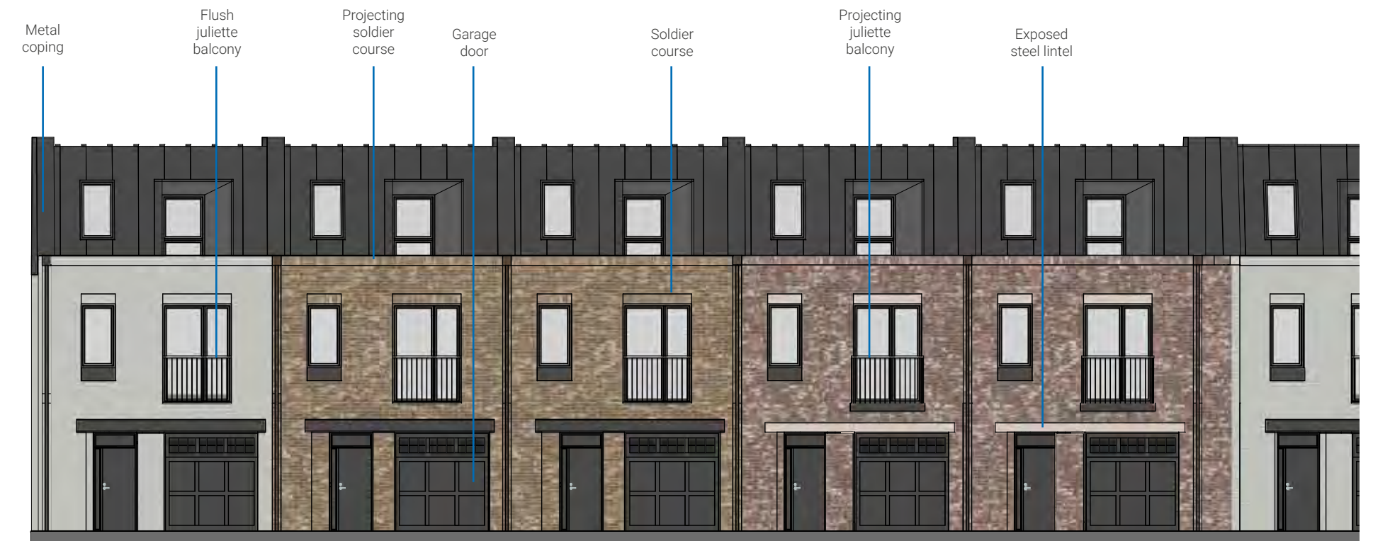
Typical west terrace elevation
