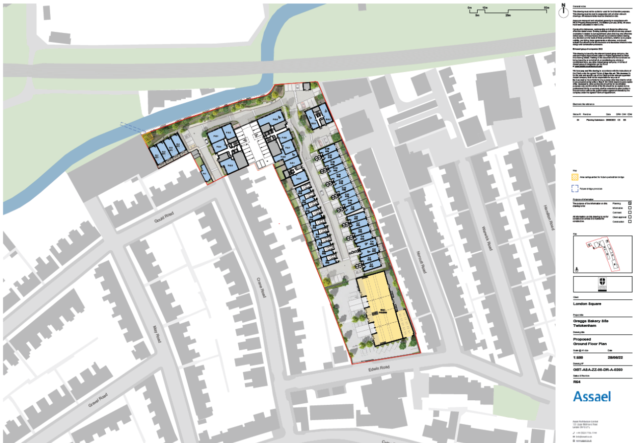
Figure ES1 Proposed Site Layout prepared by Assael Architecture (Industrial Buildings at southern end of the site)
