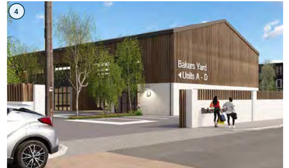
Light timber cladding with white painted brick base
