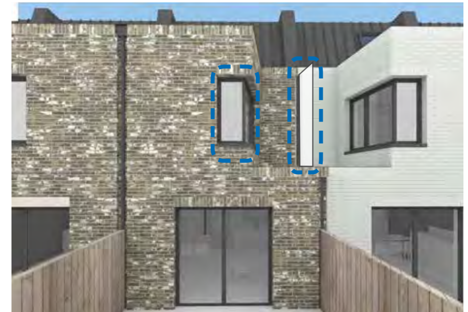
View showing the rear elevation of the east terrace houses with opaque frosted windows and privacy screen highlighted in blue
