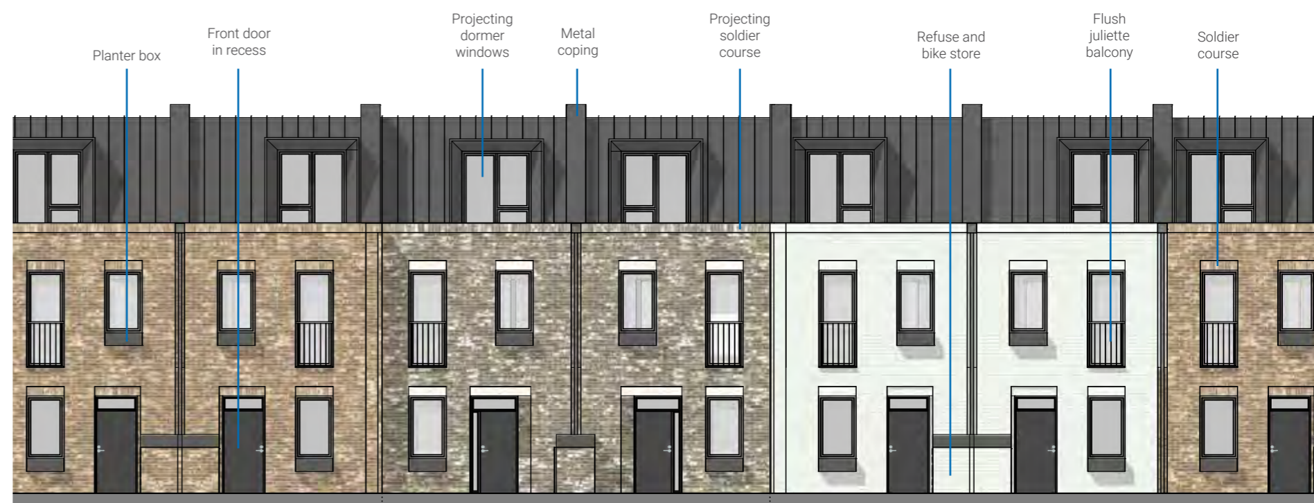
Typical east terraced houses elevation
