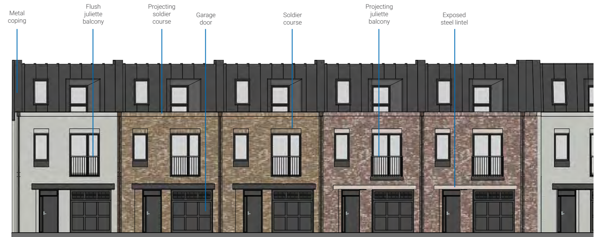
Typical west terrace elevation
