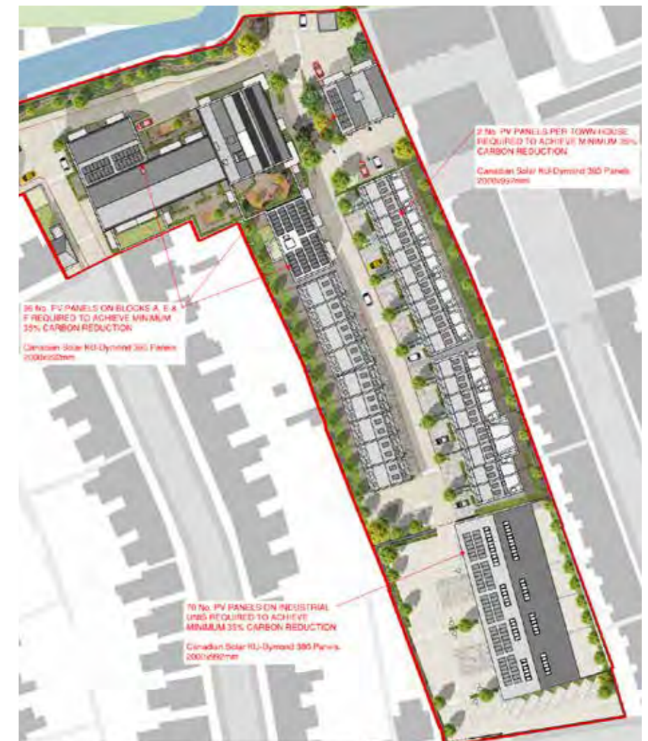
Photovoltaic panel locations
