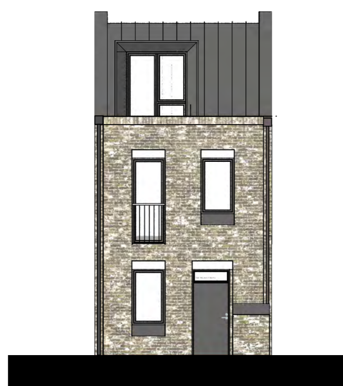
A3 Front Elevation Brown Buff brickwork Scale: 1:100
