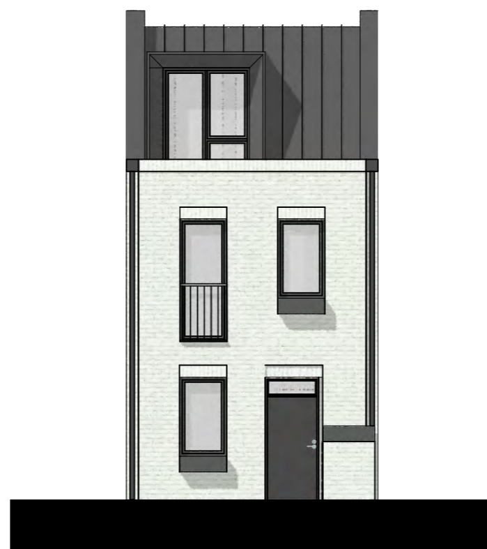
A2 Front Elevation White painted brickwork Scale: 1:100
