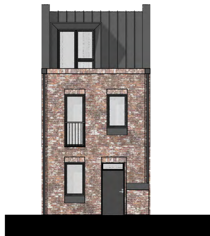
A1 Front Elevation Pink Buff brickwork Scale: 1:100
