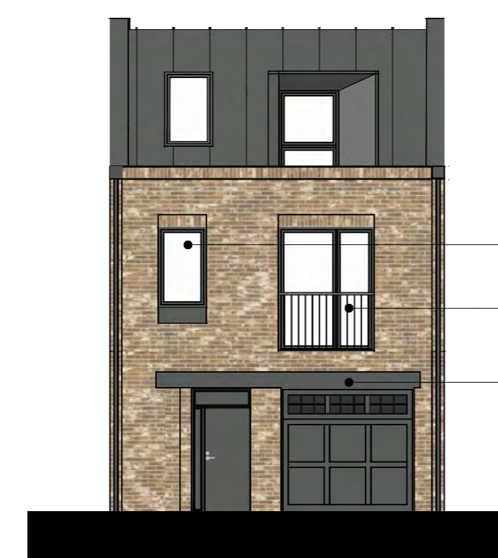
A3 Front Elevation London Stock/Multi Buff Brick Scale: 1:100
