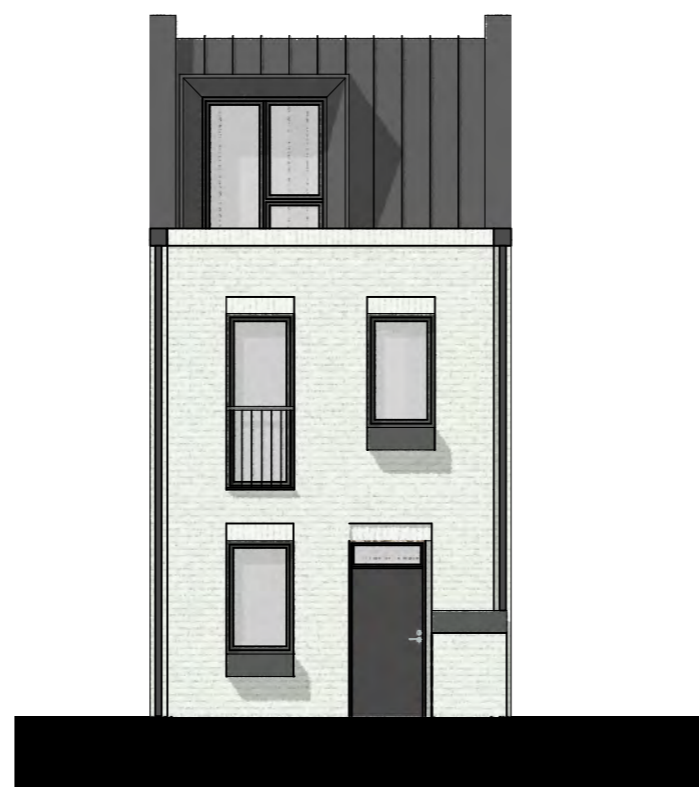
A2 Front Elevation White painted brickwork Scale: 1:100
