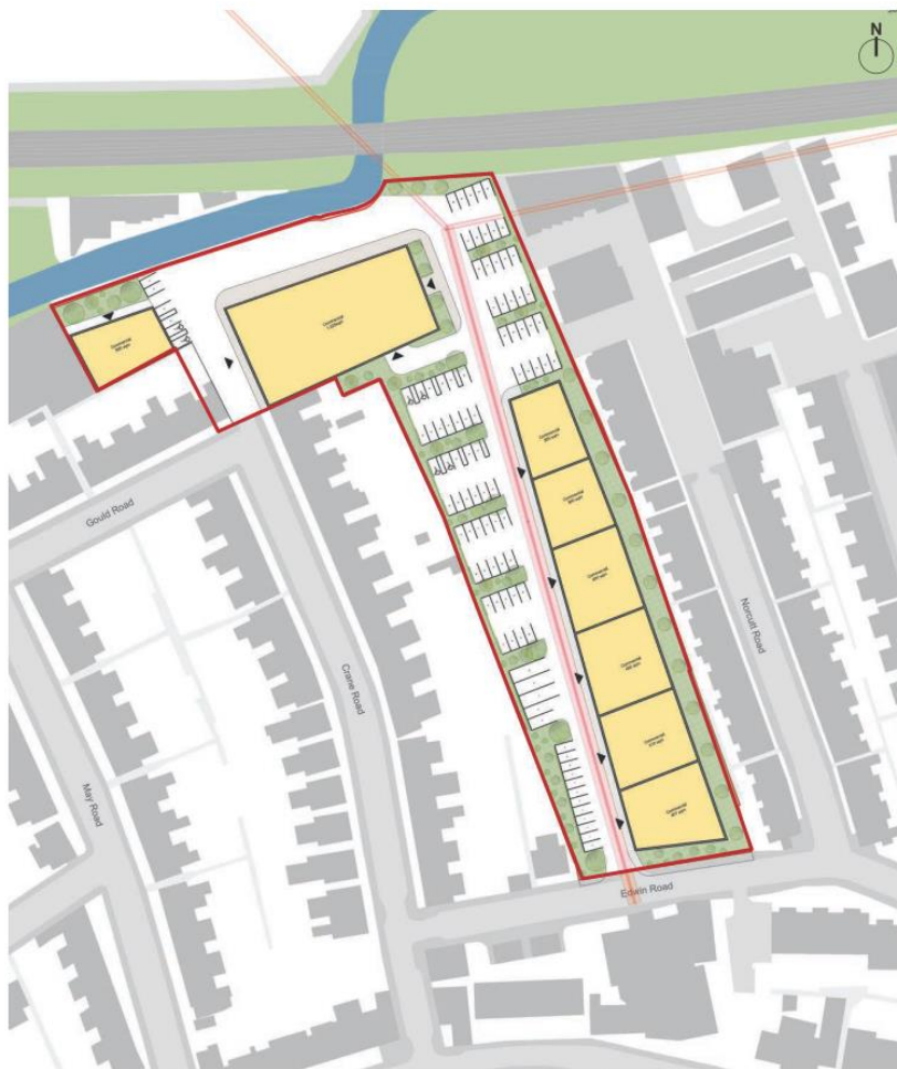
Ground floor plan of full industrial scheme of B1/B2/B8 uses achieving 3,773 sq m (1-3 storeys)
