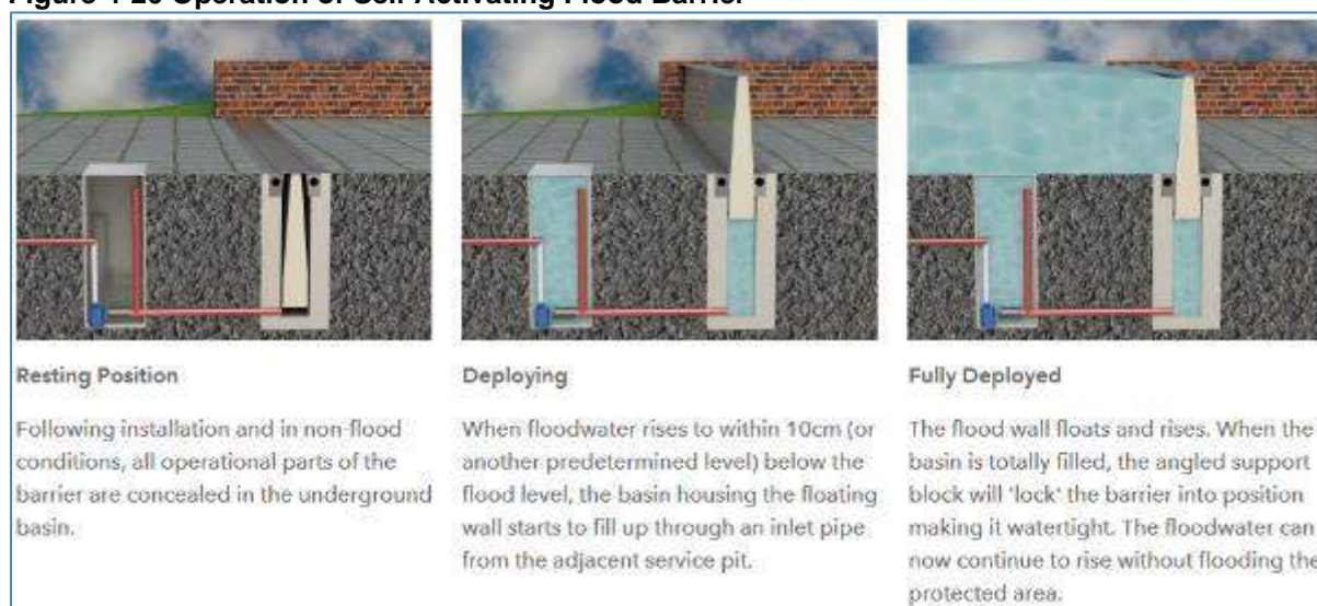
Figure 4-20 Operation of Self Activating Flood Barrier
