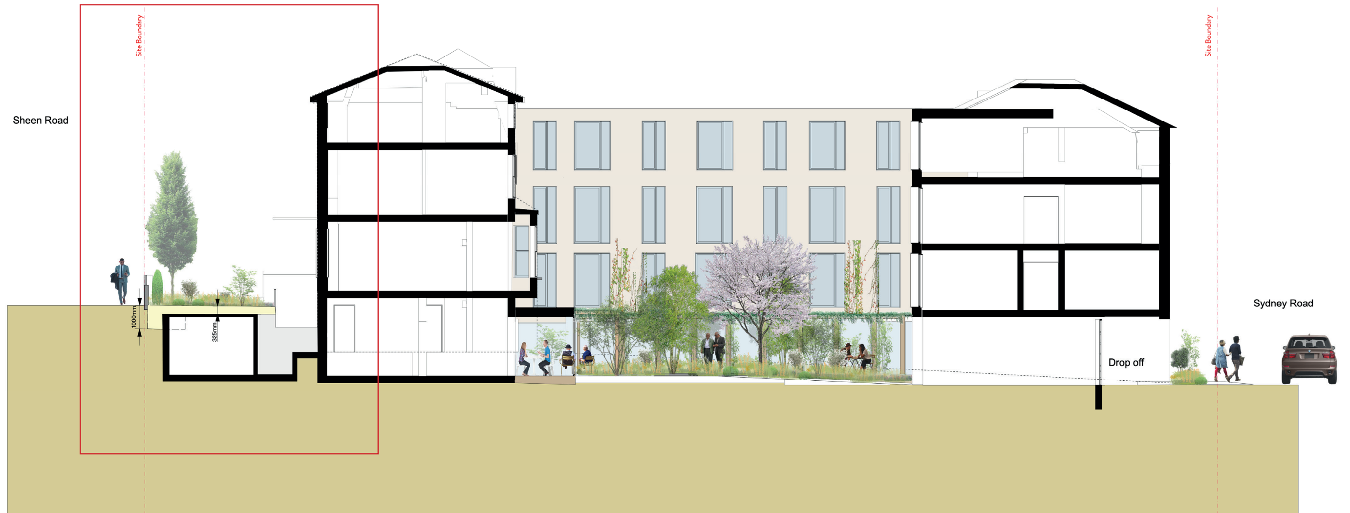
Landscape section updated to show the location and depth of the basement slab
