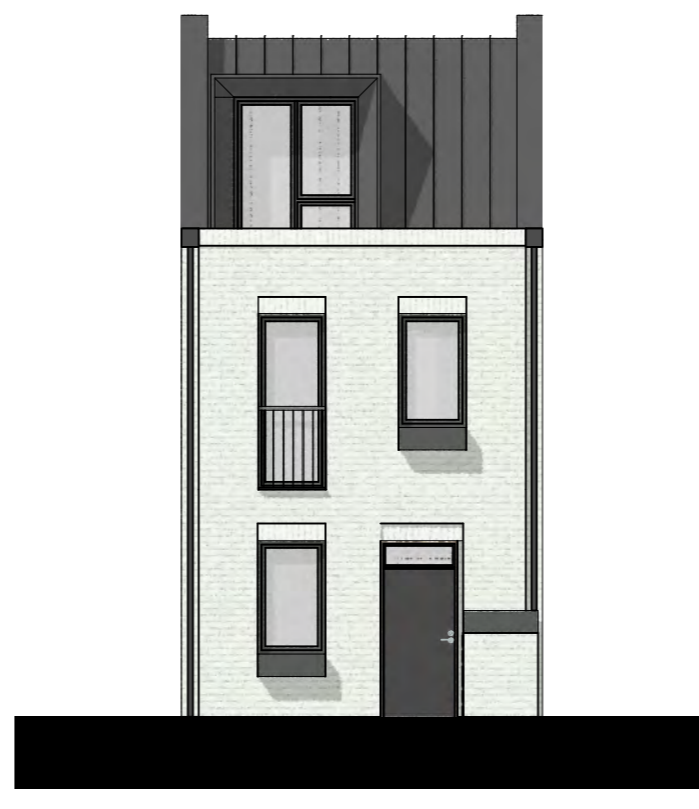
A2 Front Elevation White Painted Brickwork Scale: 1:100
