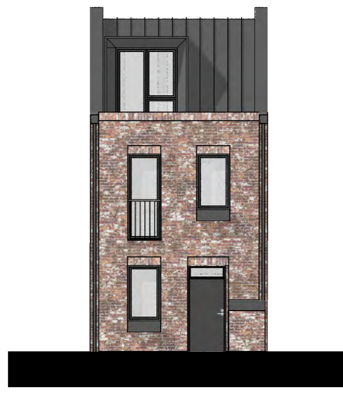
A1 Front Elevation Pink Buff Brickwork Scale: 1:100
