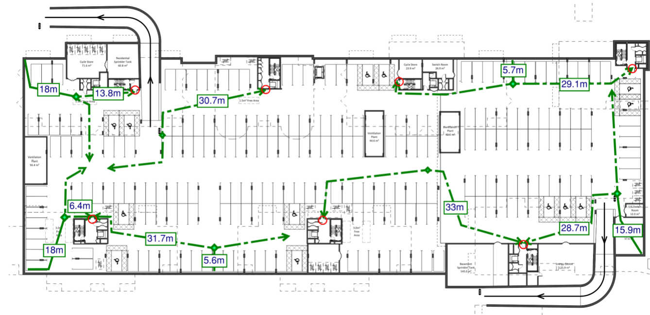
Figure 23: Means of Escape from Basement Ancillary Areas
