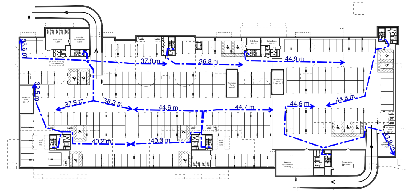
Figure 32: Hose Lay Distances - Basement Car Park
