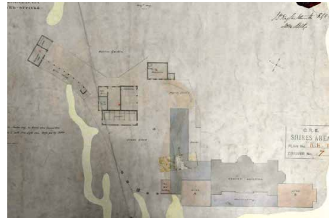
Figure 3.11 1847 site plan showing the existing building divided into its various sections and the three outbuildings to the northwest.
