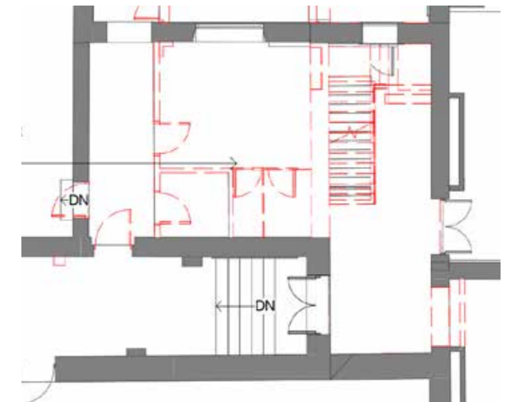
Figure 5.11 Existing plan of the staircase at ground floor level. Red = fabric proposed to be removed Drawing produced by ADP Architecture
