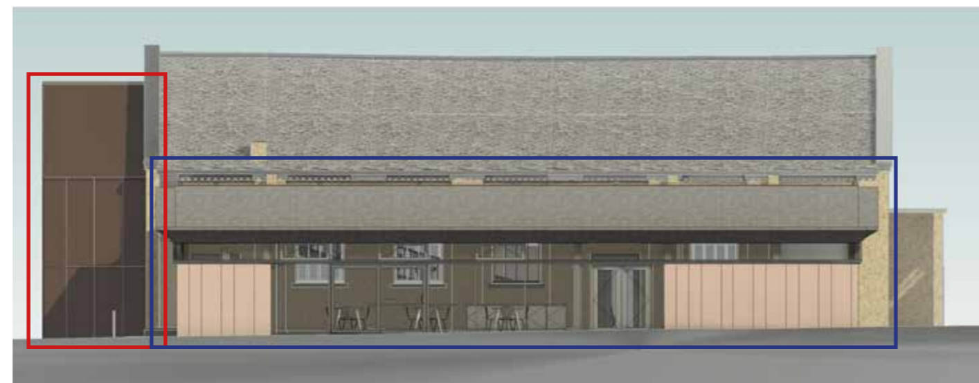
Figure 5.20 Proposed south elevation of the Band Practice Hall. Red = west addition, blue = south addition Drawing produced by ADP Architecture
