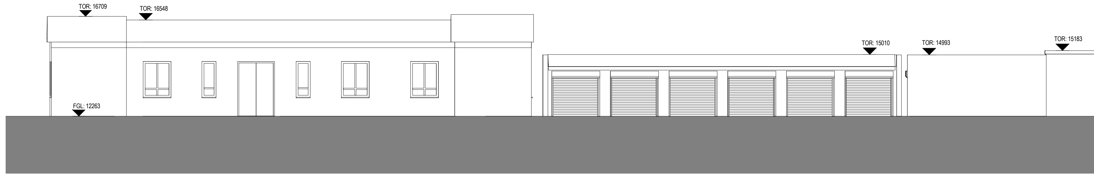
1 EXISTING SOUTH ELEVATION 1 : 100
