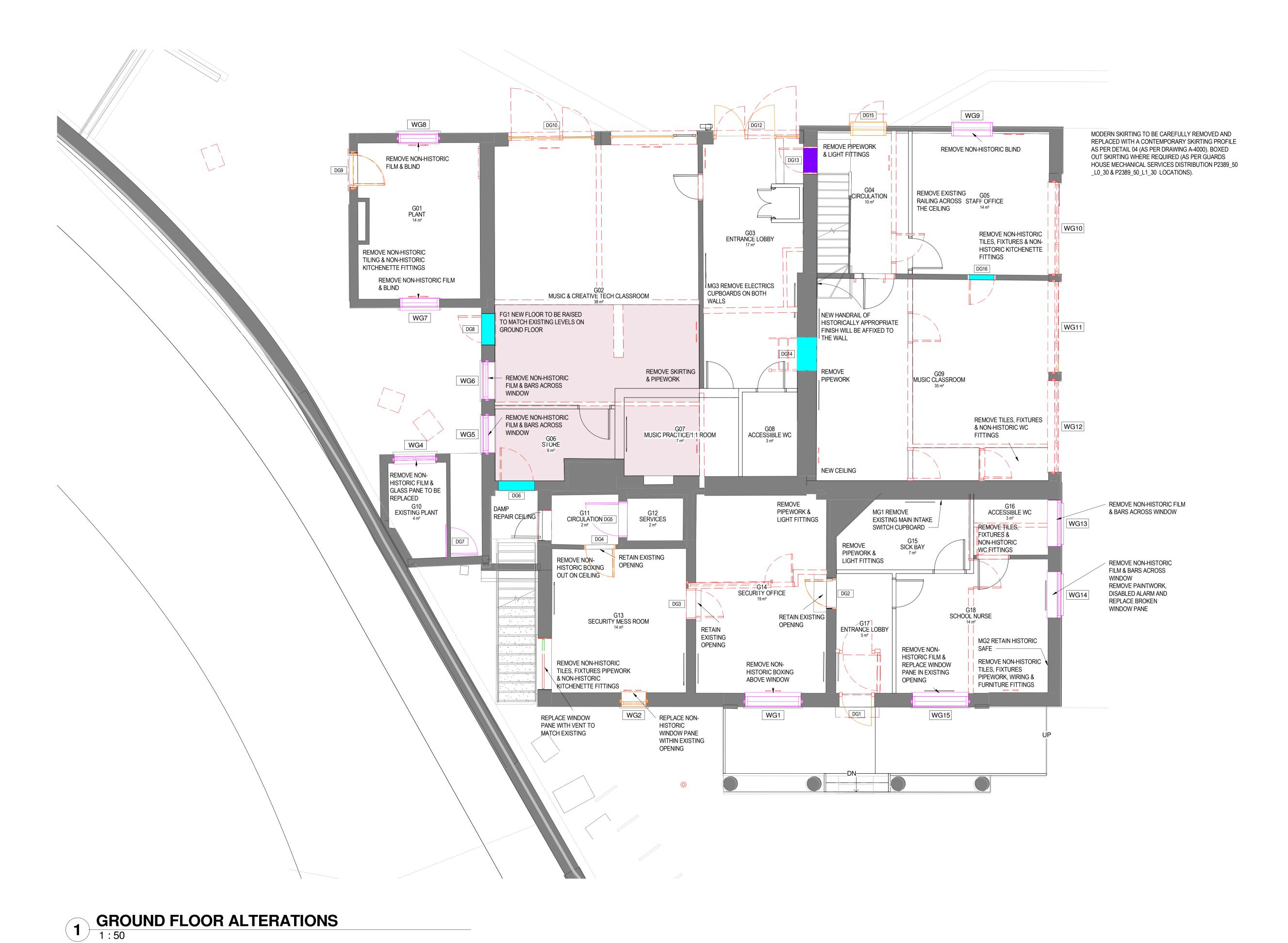
KEY REFURBISH LEAF REPLACEMENT (HISTORIC) LEAF REPLACEMENT (CONTEMPORARY) DOOR REFURBISH (FIXED/LOCKED SHUT) REFURBISH WINDOW AND REMOVE SECONDARY GLAZING REFURBISH WINDOW AND REMOVE VENT **BLOCK UP** OPEN UP RAISED FLOOR
