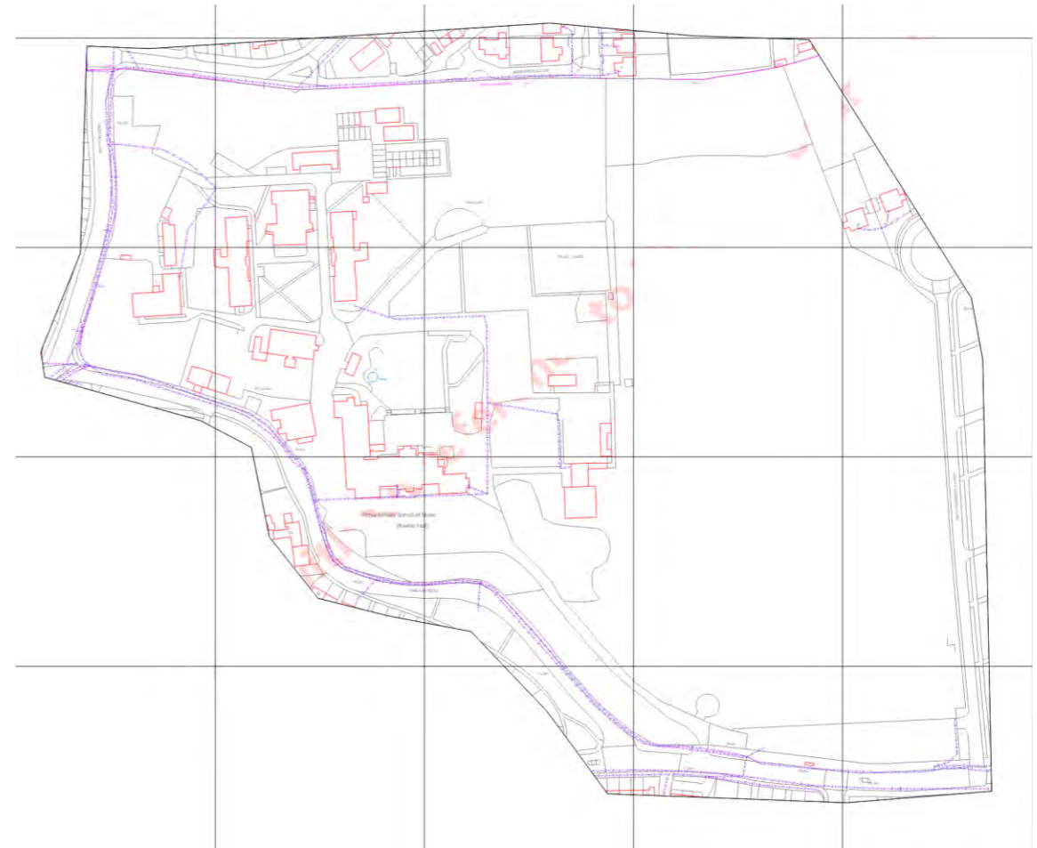
Fig 5. BT Ducts around estate perimeter
