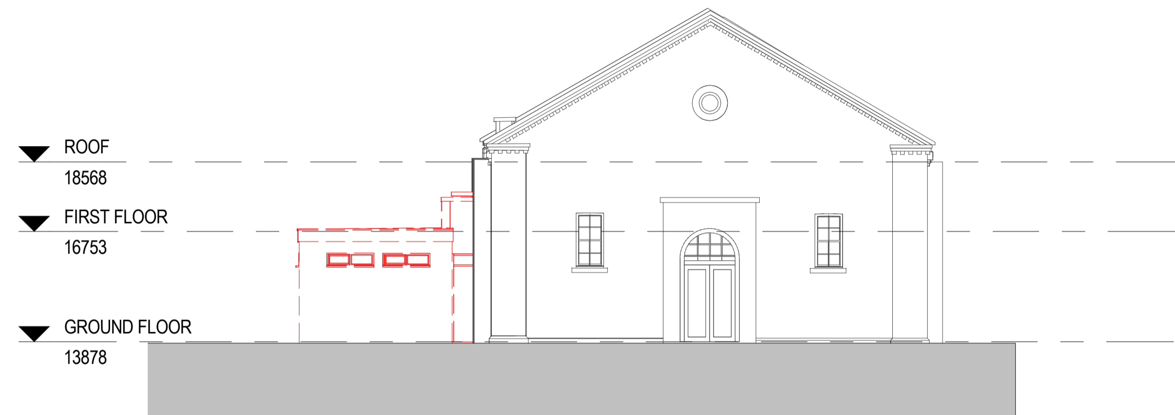
2 EAST ELEVATION - DEMOLITION 1 : 100
