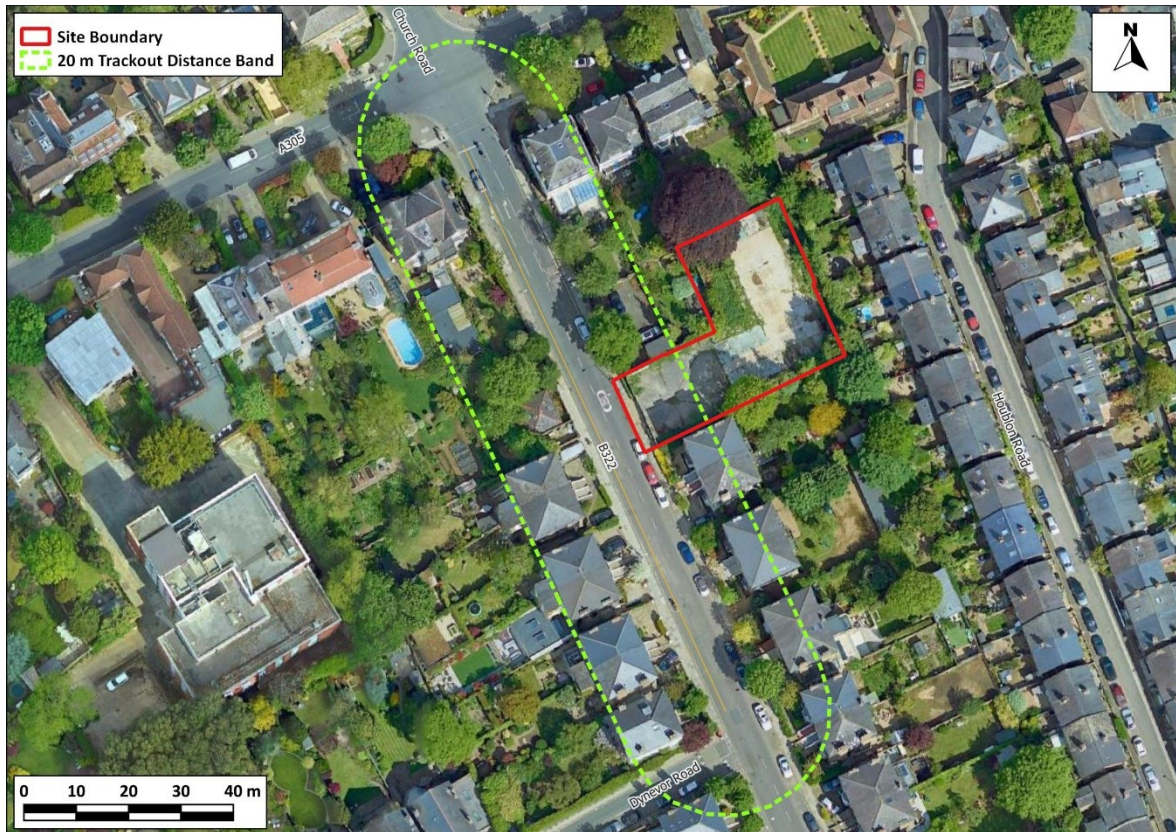
Figure 4: 20 m Distance Band around Roads Used by Construction Traffic Within 50 m of the Site Exit
