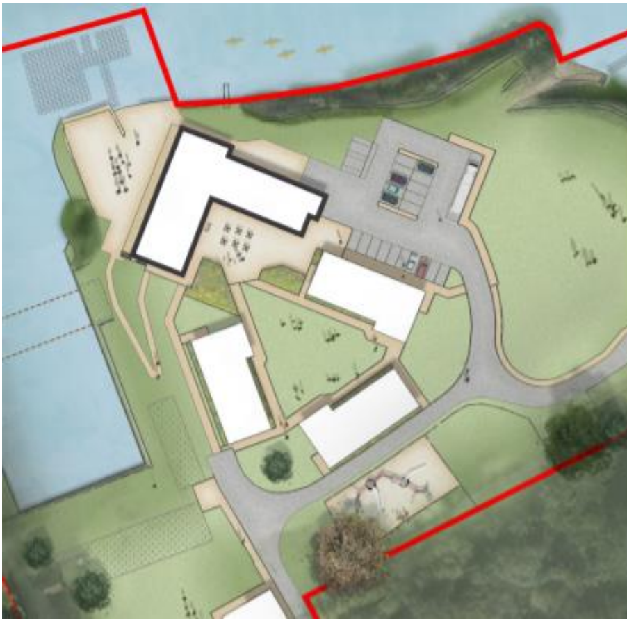
Figure 37: Block plan of the proposed main building and accommodation units, with an additional changing block to the south. Taken from Pick Everard Pre-Application Report 03, supplied by the Client.
