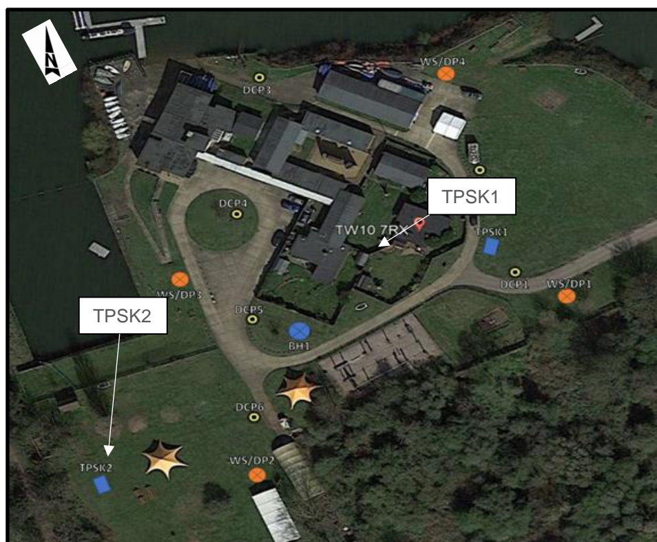
Figure 2-2 - Ground investigation locations
