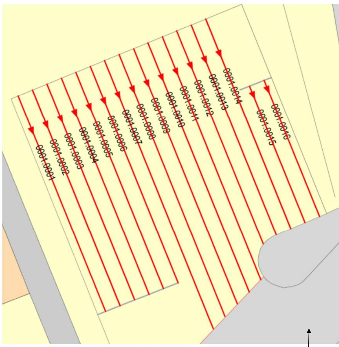
Plan 2. Extract from TreeRadar plan TRUK 0206 TR showing location of scan lines 0001.0001-0016. Do not scale.
