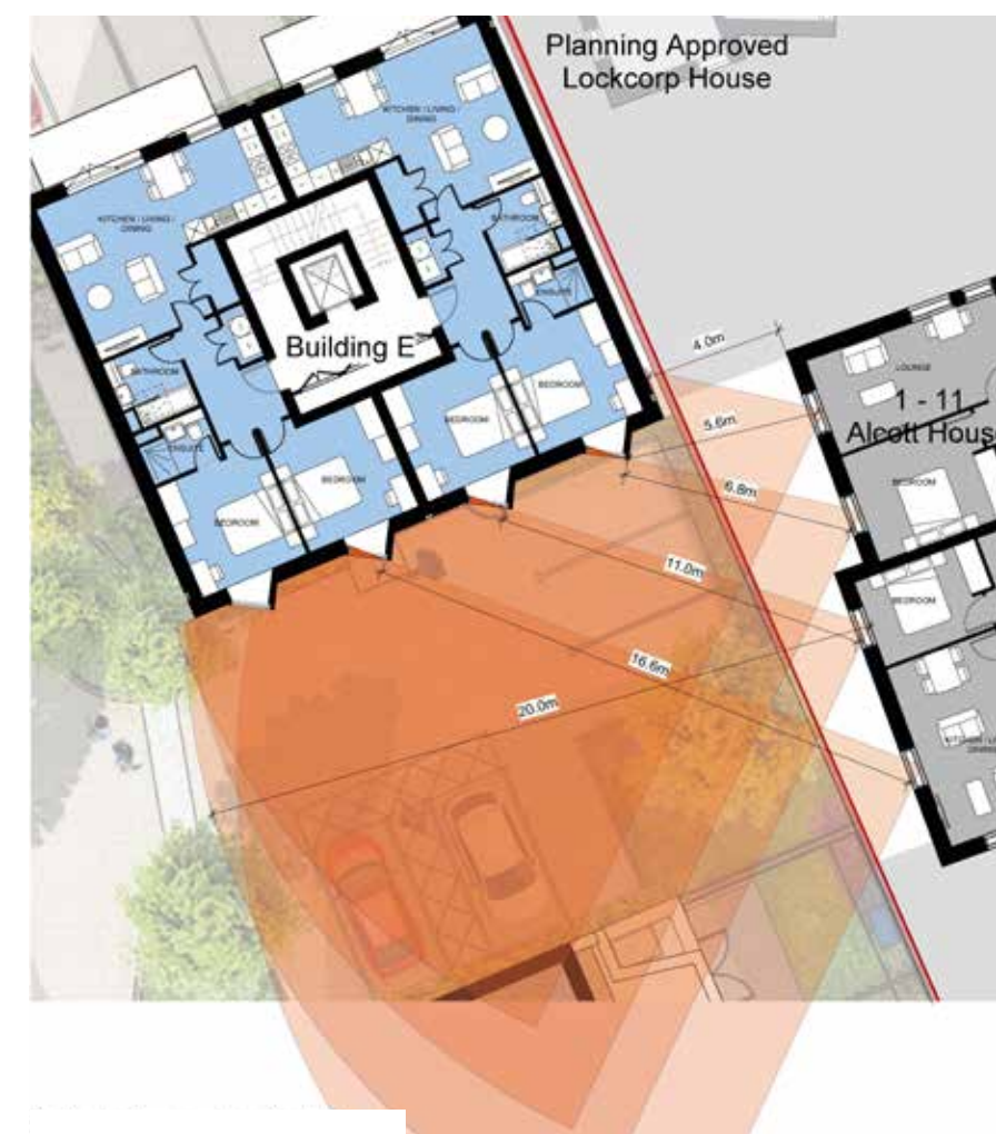
Overlooking arc from Alcott House windows showing oriel windows mitigating views from Alcott House
