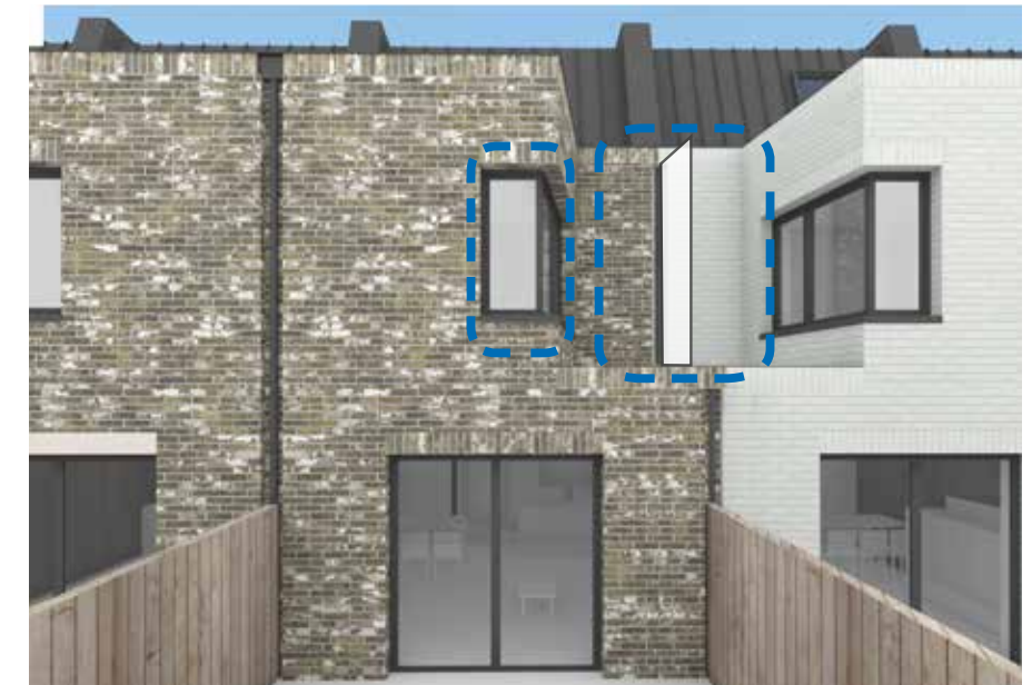
View showing the rear elevation of the east terraced houses with opaque frosted windows and privacy screen highlighted in blue
