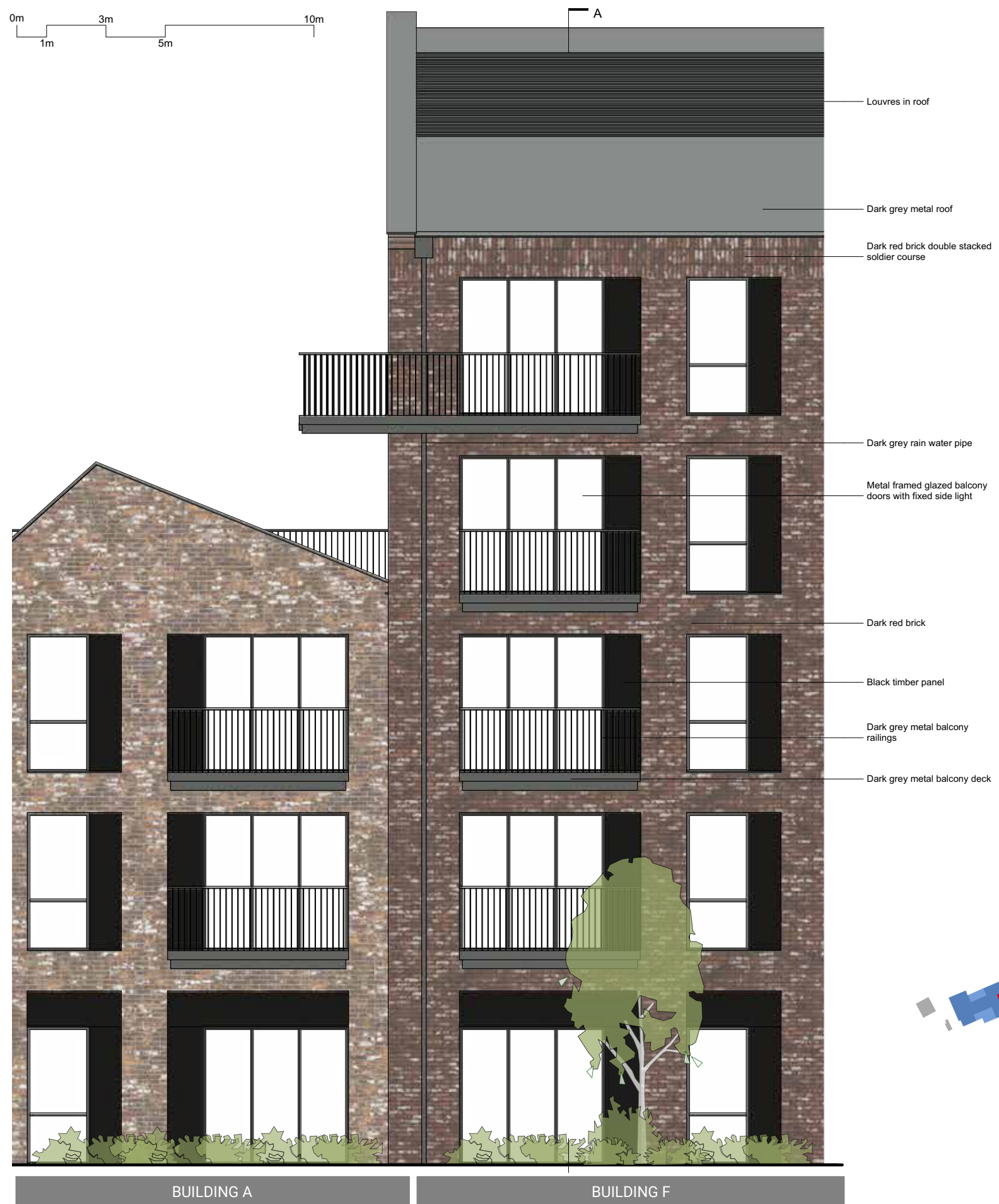
Building A and Building F east elevation showing the relationship
