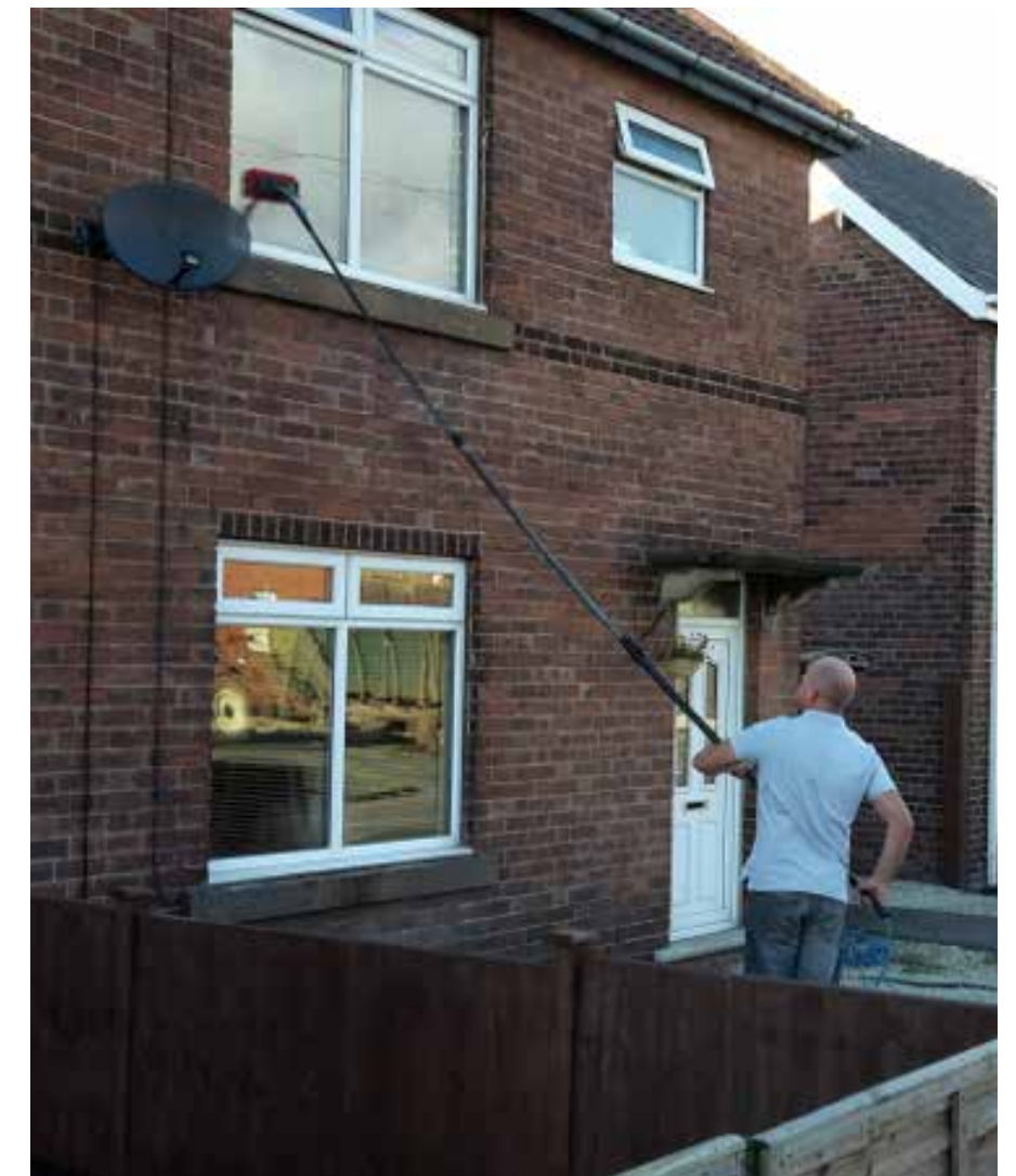
Example of long reach pole system
