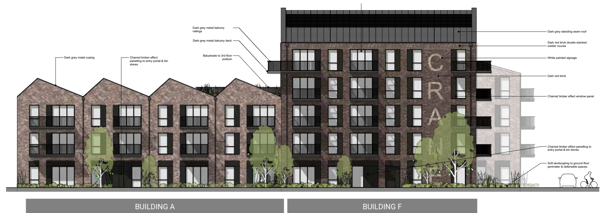
Building A and Building F east elevation
