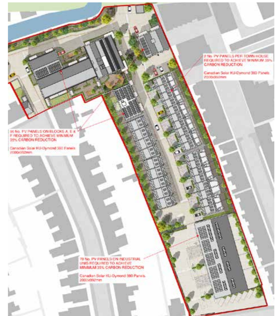
Photovoltaic panel locations
