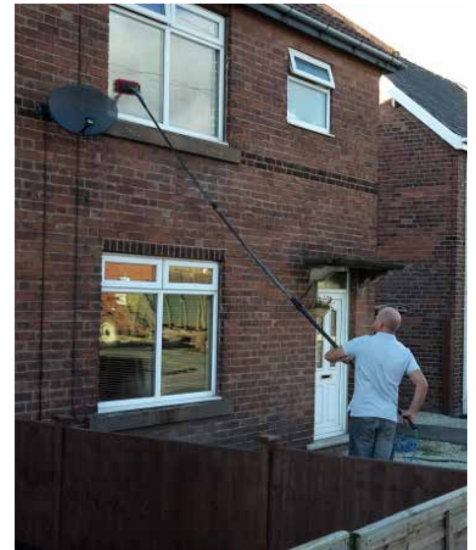
Example of long reach pole system
