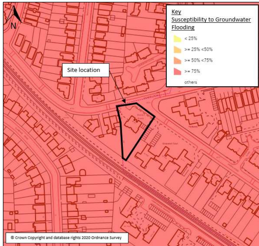
Figure 4-3: BGS Susceptibility to Groundwater Flooding
