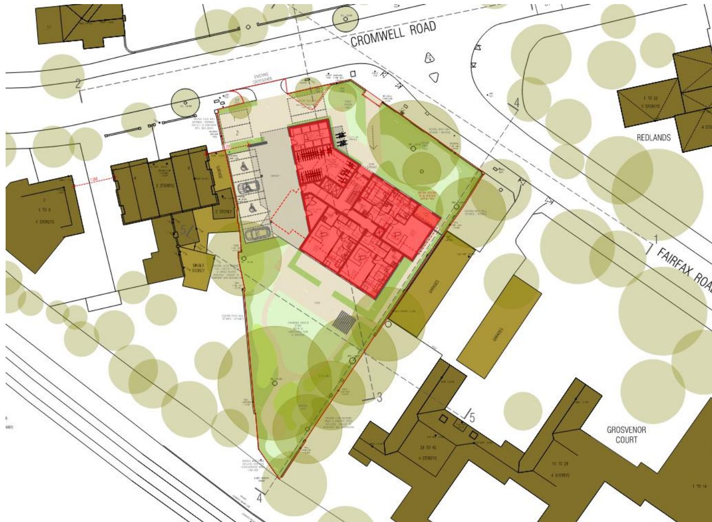
Figure 1: proposed site layout and ground floor plan of Sheldon House (Source: Clive Chapman Architects Drawing SH-03)
