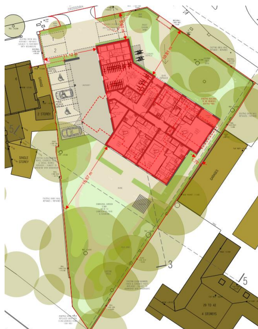
Figure 1: Proposed site layout and ground floor plan of Sheldon House (Source: Clive Chapman Architects Drawing SH-03)
