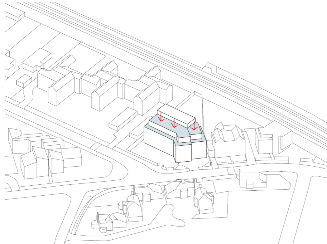
Front top floor section removed in response to overshadowing assessment to neighbouring buildings to the north along Davenport Close, and improving visual relationship with BTMs.
