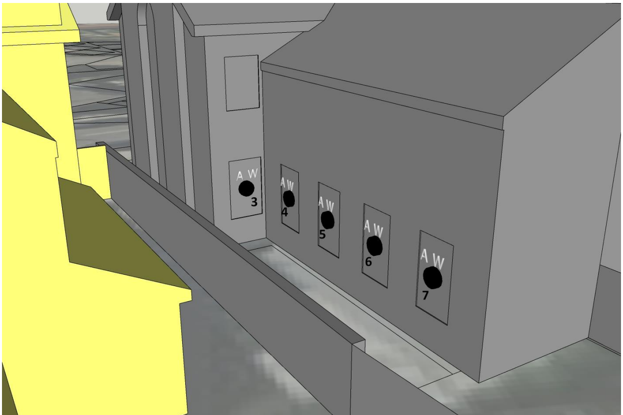
Fig 12. Rear/side view of No.64 with polycarbonate infill extension removed to show internal test points for existing windows within (note that positions of windows 4, 5, 6 and 7 are assumed due to lack of reliable survey information).
