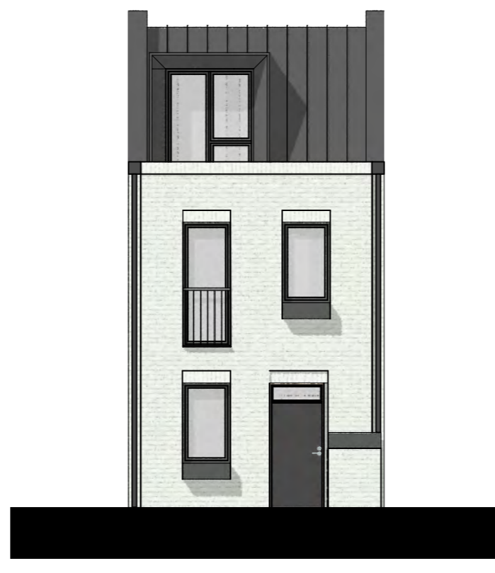
A2 Front Elevation White painted brickwork Scale: 1:100
