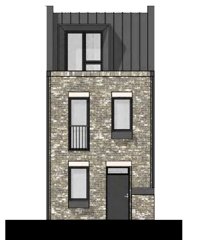
A3 Front Elevation brown buff brickwork Scale: 1:100
