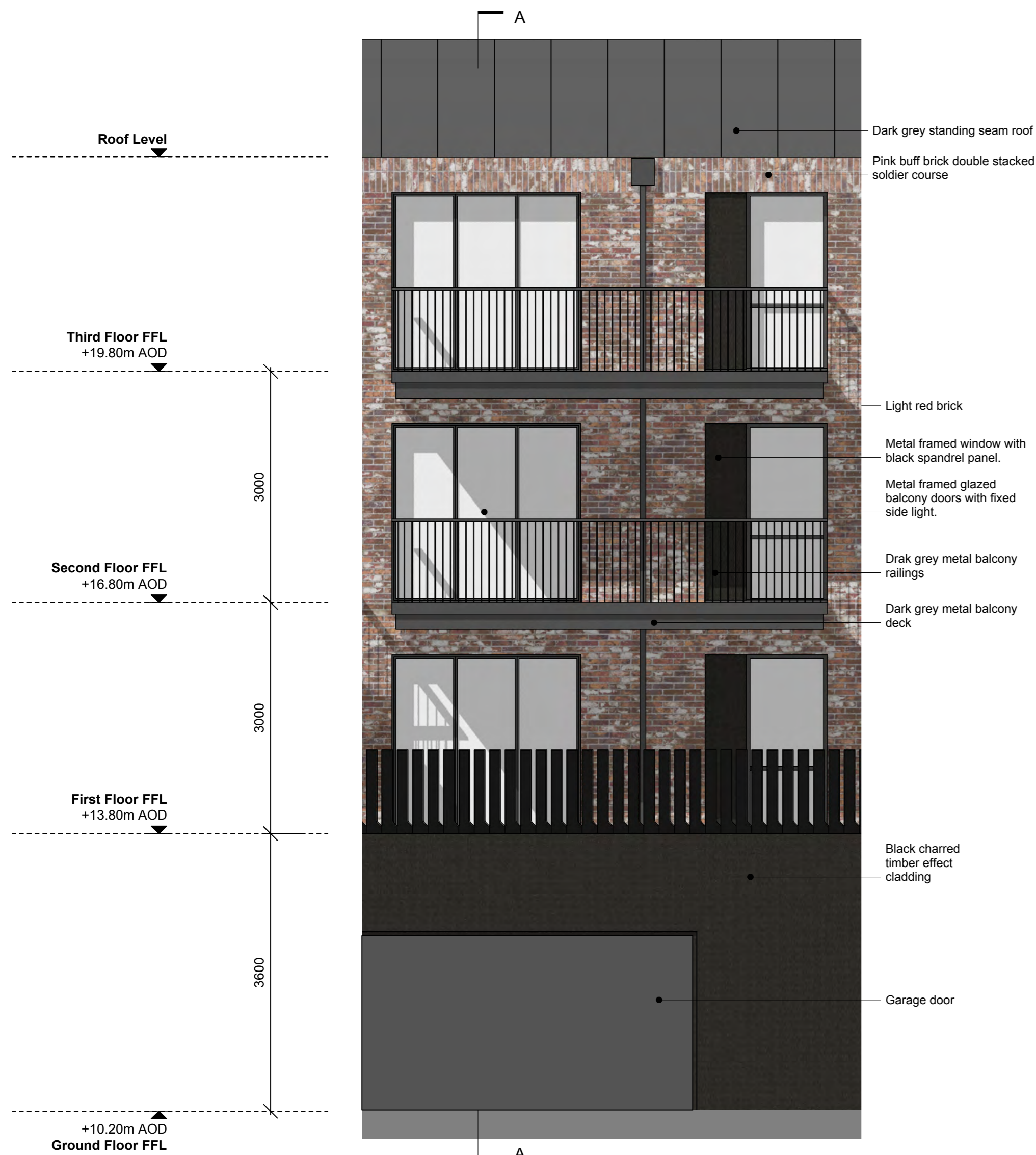
NORTH ELEVATION EXTRACT
