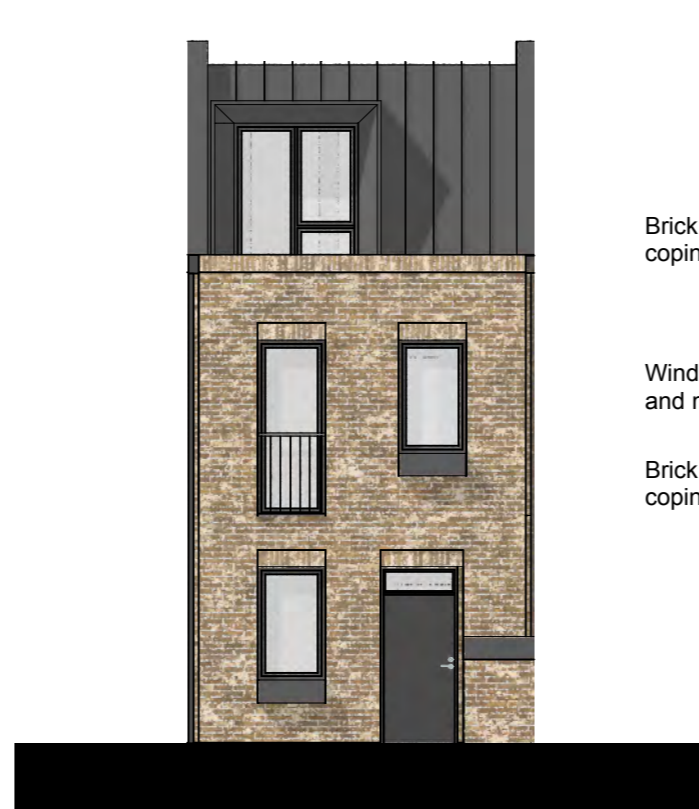
A3 Front Elevation Brown Buff Brickwork Scale: 1:100
