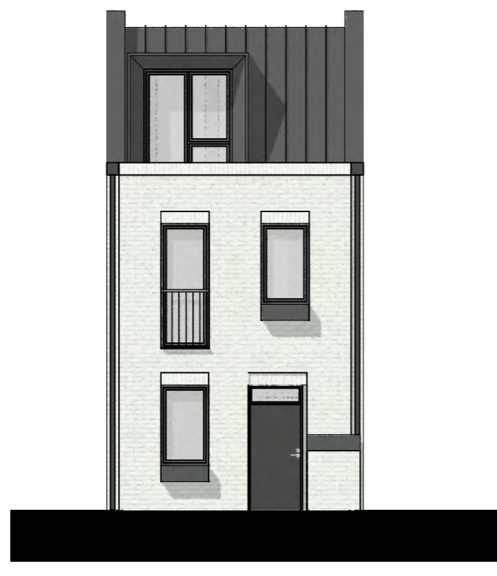
A2 Front Elevation White painted brickwork Scale: 1:100
