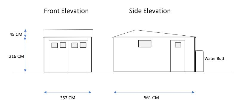
Please note that proposed roof is the same pitch, size and dimensions of the current roof. Proposed material is dark grey composite sheet in similar pattern
