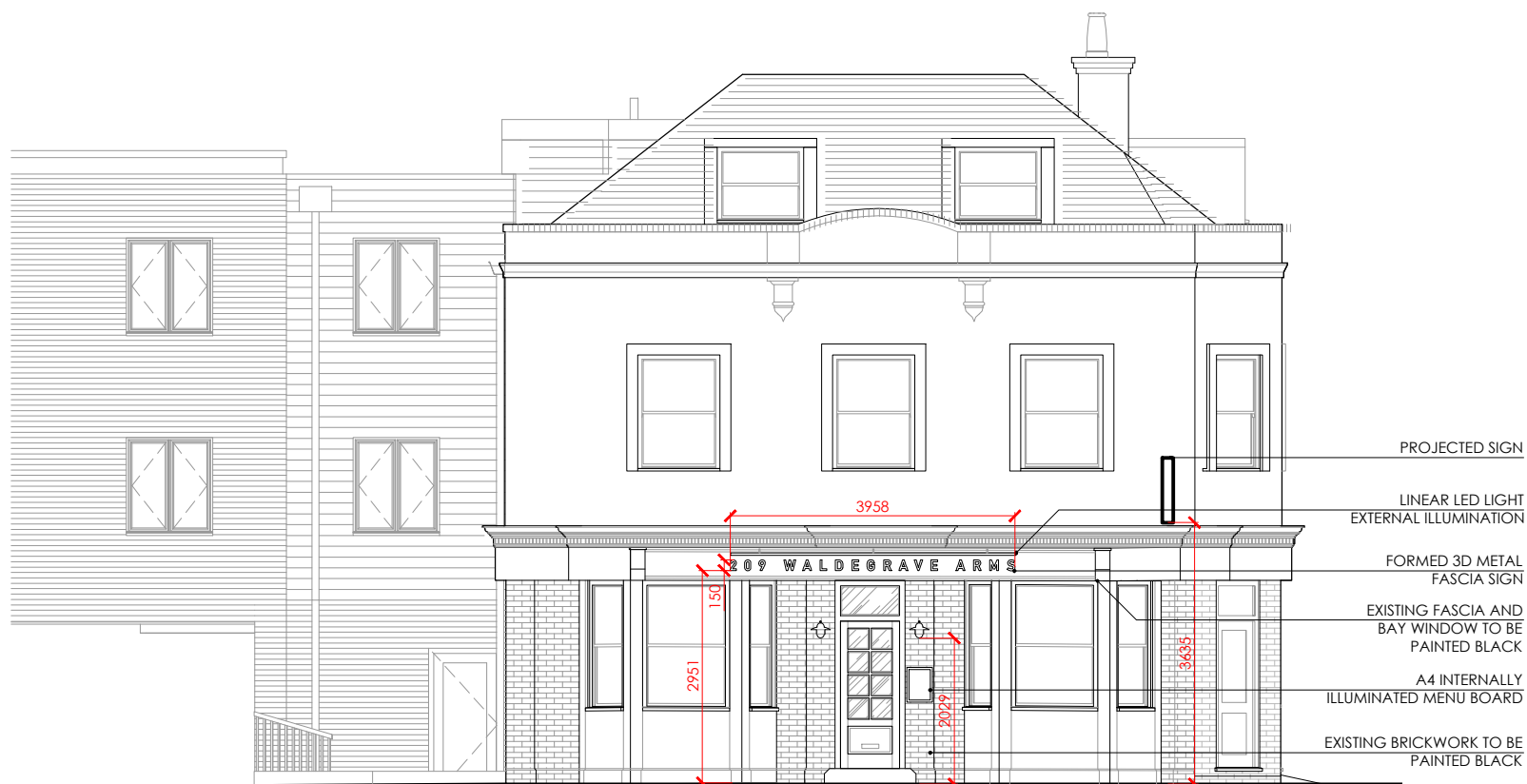
01 FRONT ELEVATION 0 1 2 3 4 5 M Scale 1:100
