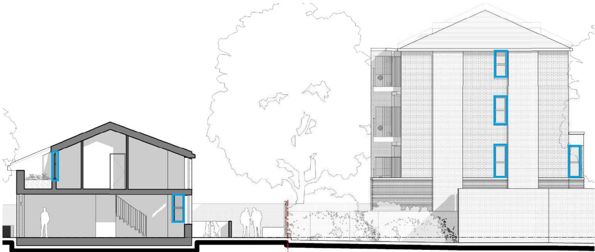
Figure 05: Glazing types (Mansion block (right) and Mews block (left), north elevation)
