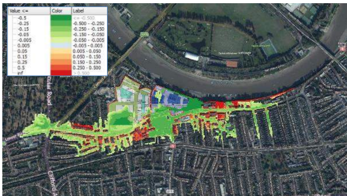
Figure D-8 Breach analysis – 2100 Baseline - Differences in depth
