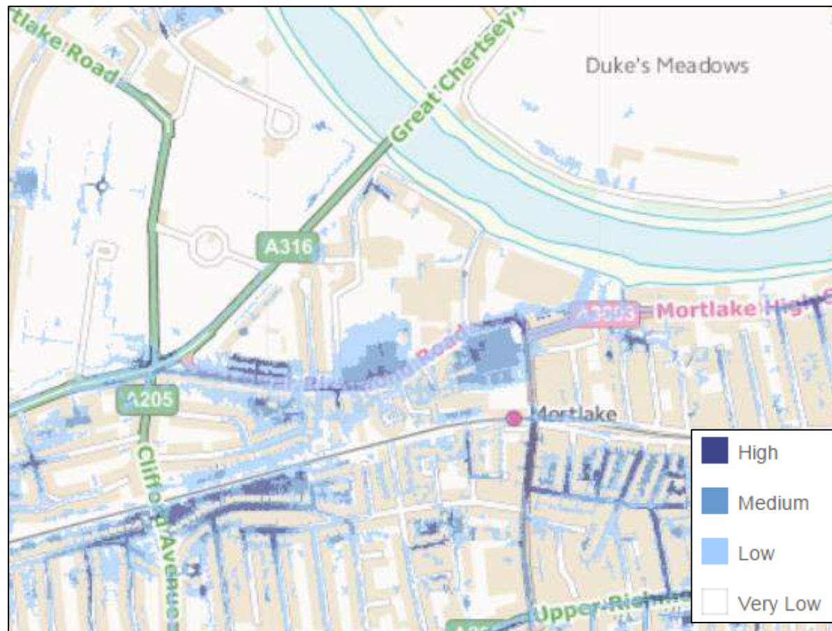
Figure 6-4 EA Areas at Risk of Surface Water Flooding
