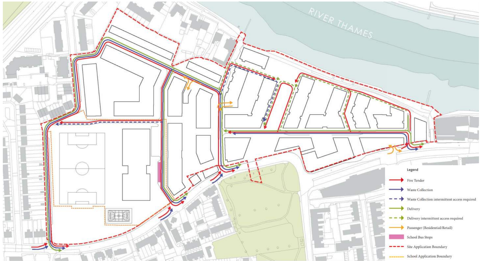
Figure G-1 On-site Access Route
